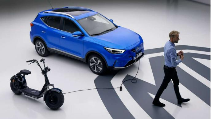
The handy V2L (vehicle-to-load) reverse charging function extends the utility of the battery pack. Connect external devices like an electric barbecue, cooling box or e-bike and power them off the car's own battery. It's like having your own portable power station.
