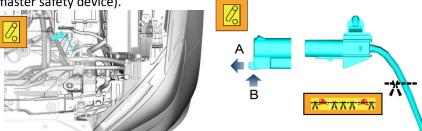
Open the bonnet, pull out the clip the manual service from disconnect(A), press the end of the clip (B) and remove the manual service disconnect.
